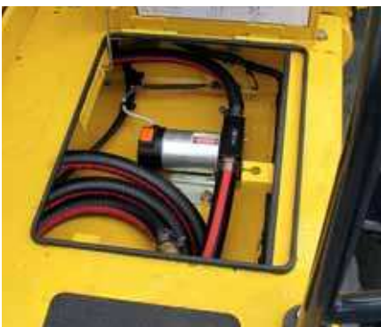
Electric refuelling pump
